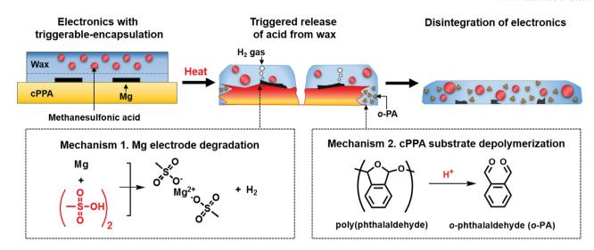
Figure 1. Heat-triggerable transient electronics coated with wax containing acid dispersions. Release of MSA by melting a wax coating leads to rapid electronic destruction by acidic degradation of Mg electrodes on glass. In addition, using a cyclic poly(phthalaldehyde) (cPPA) substrate affords a more rapid destruction of the device due to acidic depolymerization of cPPA.
